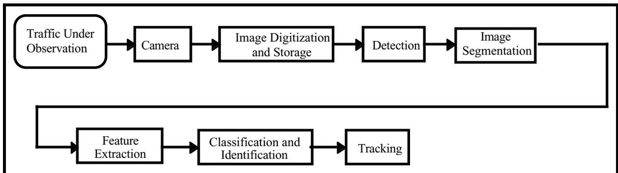
**Figure 17. Conceptual image processing for vehicle detection, classification, and tracking.**
