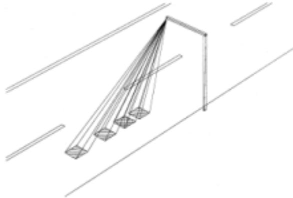
**Figure 28. Multiple detection zone configuration in a passive infrared sensor.**
