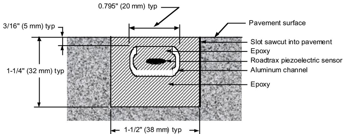
**Figure 6. Roadtrax piezoelectric BLC sensor mounted in aluminum channel as installed in a roadbed (Roadtrax, 1995-1996).**
