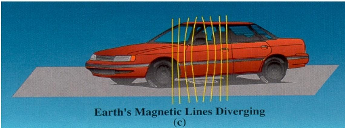
**Figure 8.** Distortion of Earth's magnetic field created as a vehicle enters and passes through the detection zone of a magnetic sensor. (Drawing courtesy of Nu-Metrics, Vanderbilt, PA).
