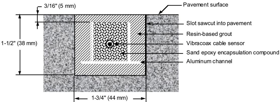
**Figure 5. Vibracoax piezoelectric sensor mounted in aluminum channel as installed in a roadbed. (Drawing courtesy of IRD, Inc., Saskatoon, SK).**
