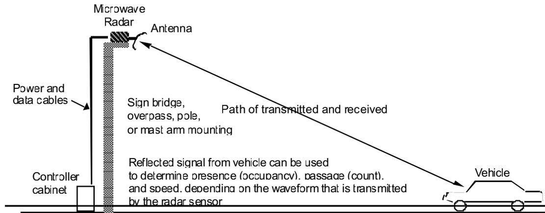
**Figure 19. Microwave radar operation.**
