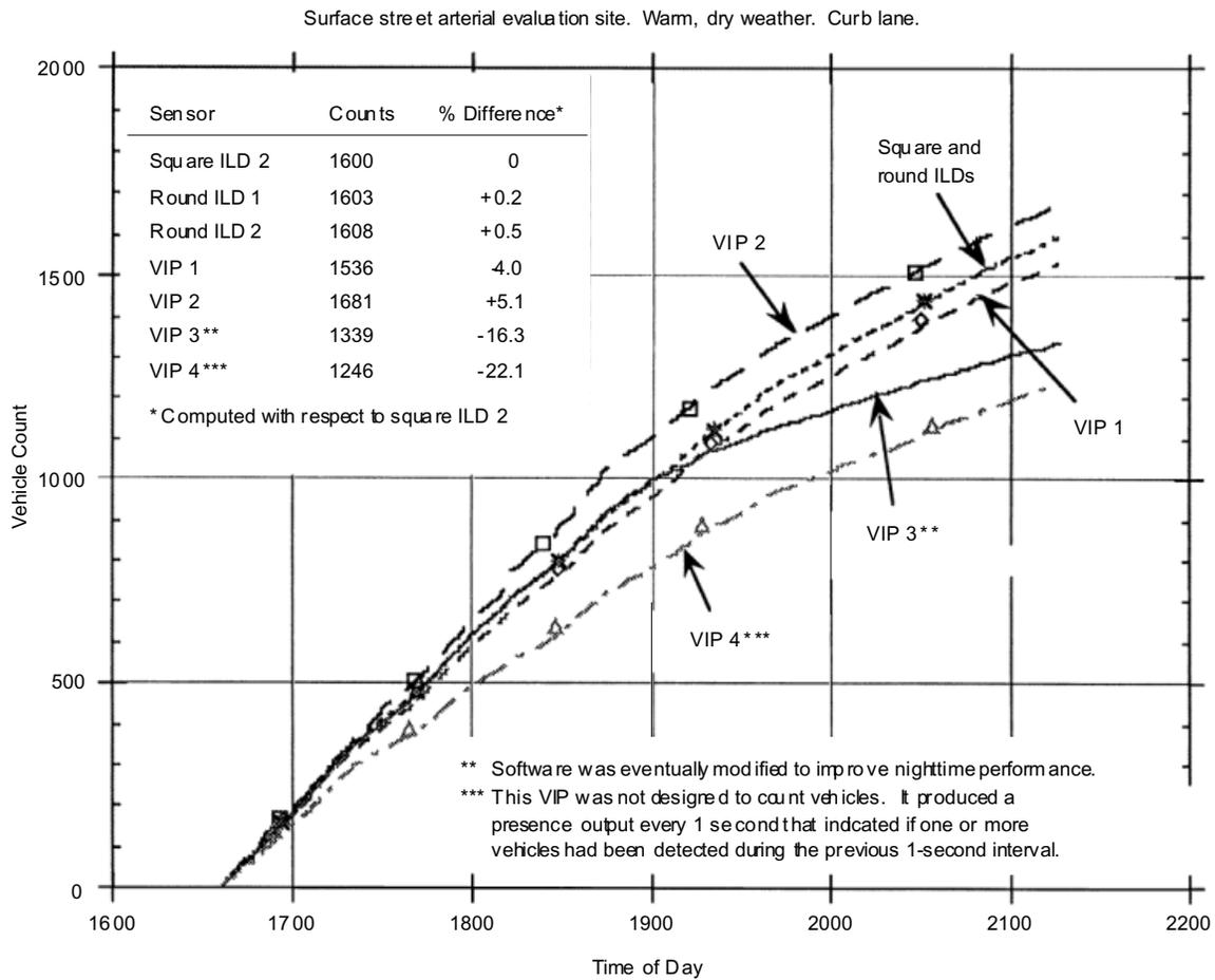
**Figure 18. Vehicle count comparison from four VIPs and inductive loop detectors.**
