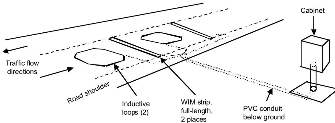
**Figure 13. WIM installation with full-length piezoelectric sensors.**
